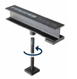
The two-piece steel bearing variant is not supplied preassembled due to the more favourable space requirement during transport. Steel support and anchoring bar are packed separately here. Therefore, the anchoring bar with anchor plate must be screwed into the socket of the steel profile prior to the installation of the steel bearing in the formwork. The tightening torques given in Table 1 must be observed when doing this.
